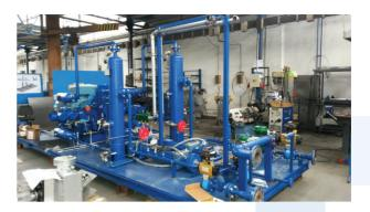
5,000 kW for raw natural gas, pipeline gas, CO2 and nitrogen. Based on the request of our partners our devices can be **fix or mobile units**. As a manufacturer independent system designer and manufacturer, we build our equipment using the most suitable elements for the job reciprocating, rotary vane or screw.
