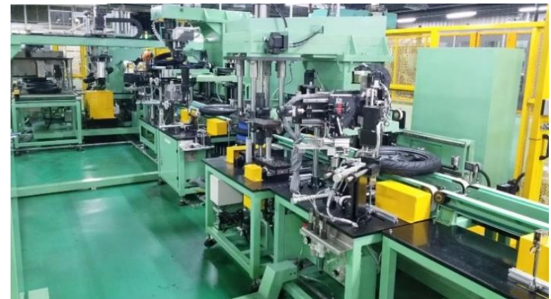
Automatic Wheel Mounting Line with Robots
